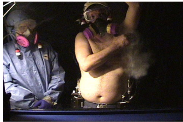
Figure 4 Application with powder puff in bathroom-sized chamber.
